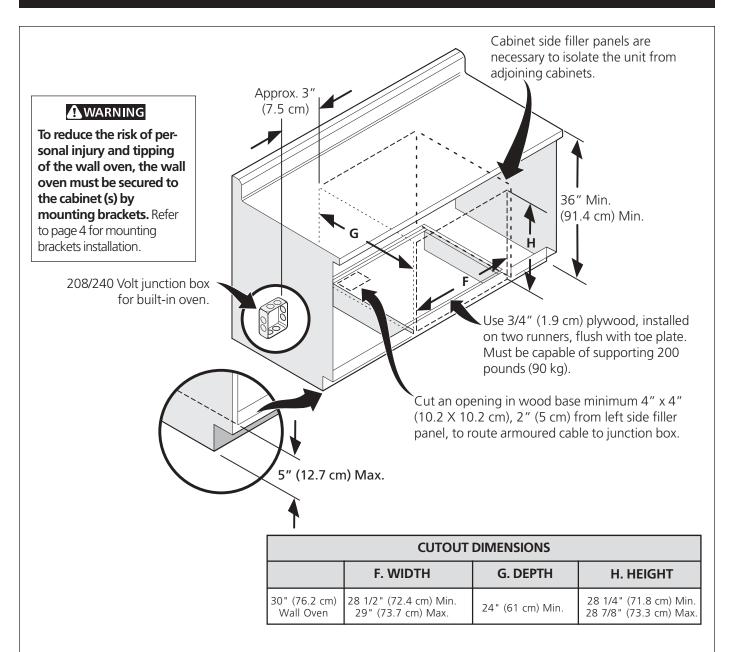
Figure 8- TYPICAL UNDER COUNTER INSTALLATION OF AN ELECTRIC BUILT-IN OVEN
